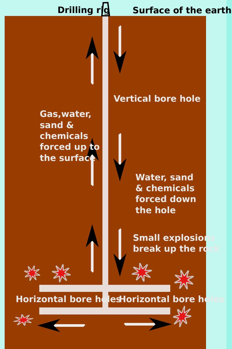
Fracking has been widely used for many years to produce oil. It's now being used to extract shale gas in many areas of the world.
