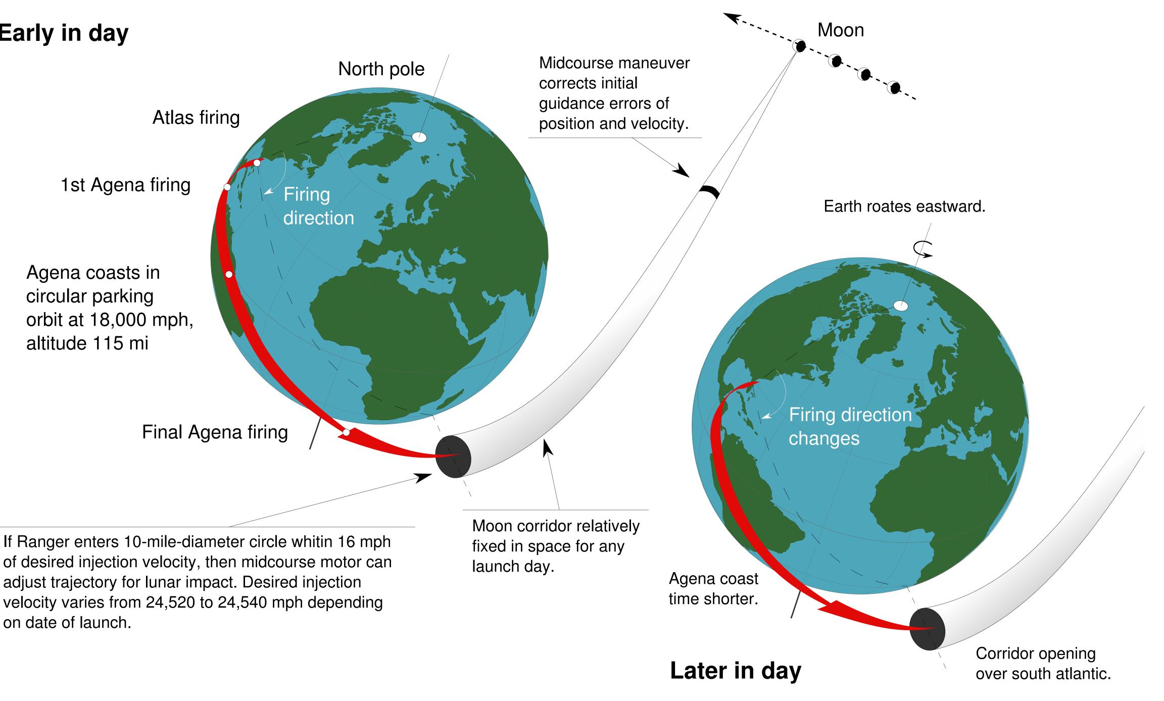
of desired injection velocity, then midcourse motor can adjust trajectory for lunar impact. Desired injection velocity varies from 24,520 to 24,540 mph depending on date of launch.
