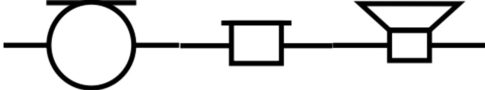
Microphone: 1-2. Common. 3. Condenser. 4. Piezoelectric.
